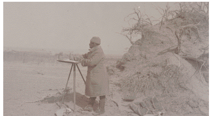
Stein at his plane table surveying the Taklamakan desert on his 3rd expedition, March 7, 1915
